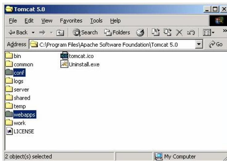
Apache Tomcat is configured with the following program files: `\conf\server.xml`, `\conf\web.xml` and `\webapp\Carpool\WEB-INF\web.xml` (the second web.xml file is used to declare servlets for web access for security reasons and is required because the connection pool manager used in the application is partially declared in the file. Connection pool
