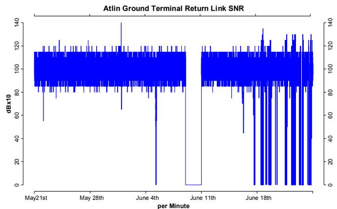
Fig. 2. Return link SNR recorded per minute at ground terminal location Atlin from May 21<sup>st</sup> to June 24<sup>th</sup>, 2007
