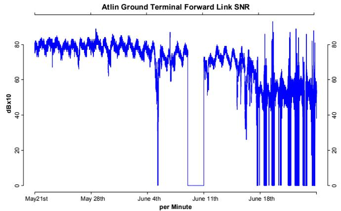
Fig. 1. Forward link SNR recorded per minute at ground terminal location Atlin from May 21<sup>st</sup> to June 24<sup>th</sup>, 2007
