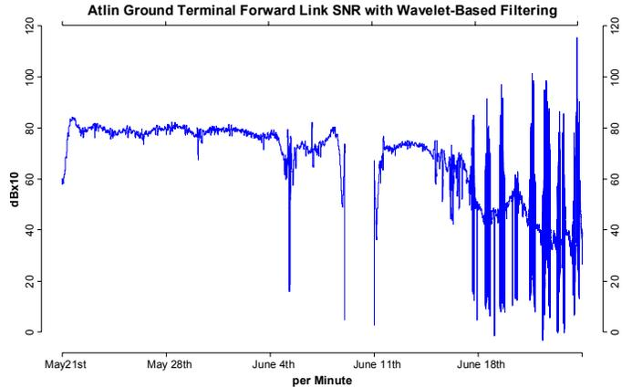
Fig.4. Inverse MODWT over the resulting wavelet and scaling coefficients from Fig.3. Periodic trend was smoothed out at wavelet coefficient level 10, and noise terms were removed from wavelet coefficient level 1 to 4.
