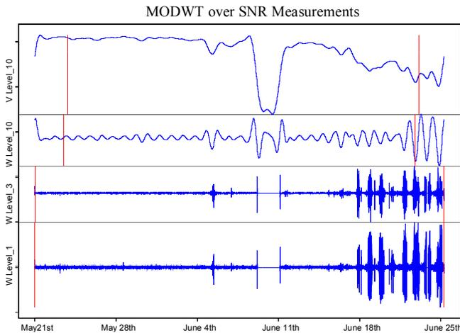
Fig.3. MODWT over SNR plotting in Fig.1 with D(8) wavelet filter and maximum level  $J=10$ . Selected wavelet coefficient level 1, 3, 10 and scaling coefficient level 10 are plotted from bottom to up. The red lines distinguish out the boundary coefficients at sides.
