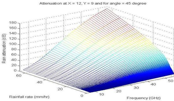
Fig. 5. Rain Attenuation – Function of Frequency and Rainfall rate
