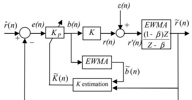
Figure 10. Linearized system block diagram with adaptive  $P$  controller.
