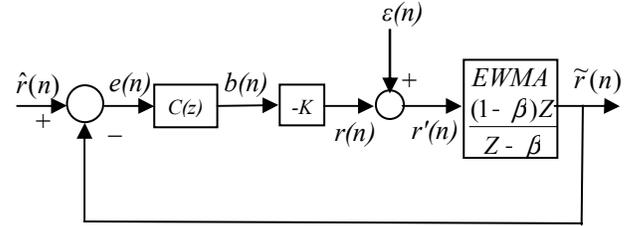
Figure 2. Linearized system block diagram.
