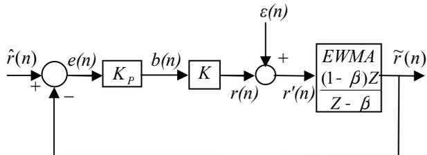
Figure 4. Linearized system block diagram with simple  $P$  controller.
