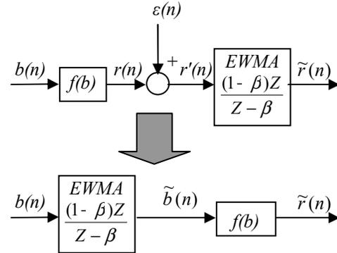
Figure 9. Equivalent transform of part of the system.
