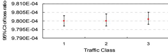
Fig. 4 95%CI of loss ratio with AEBA under DWRR
