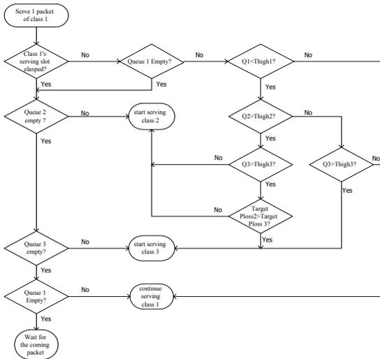
Fig.2 DWRR with buffer overflow preventive mechanism
