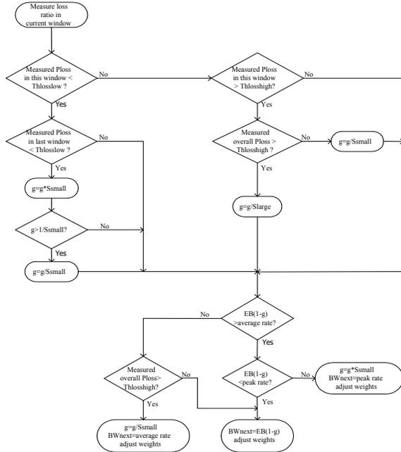
Fig.3 Adaptive effective bandwidth allocation
