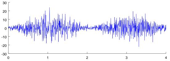
An example EMG signal (mV vs. time (s)) from a muscle which is active at two different episodes
