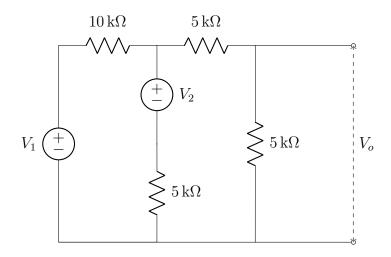
In the circuit above,  $V_1$  is 1 V, and  $V_2$  is 2 V.
