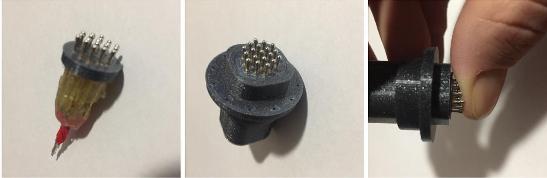
**Figure 4.2:** Left: Probe array without casing showing internal electronics. Middle: Probe array without casing showing the mounting assembly. Right: Demonstration of probe array spring loading and contact quality on uneven surfaces.
