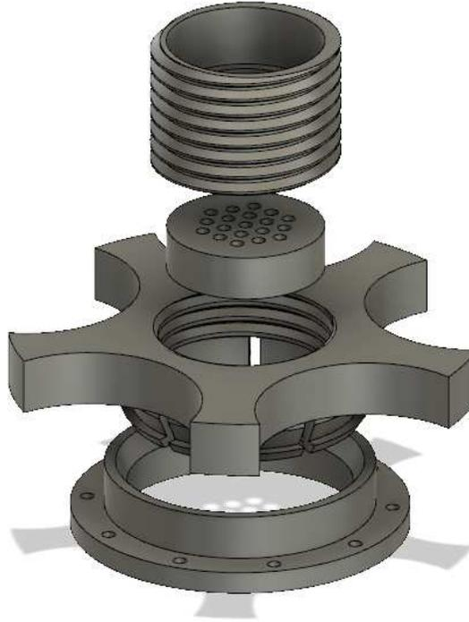
**Figure 4.11:** Proposed electrode design with rotating electrode housing that allows for scalp abrasion.
