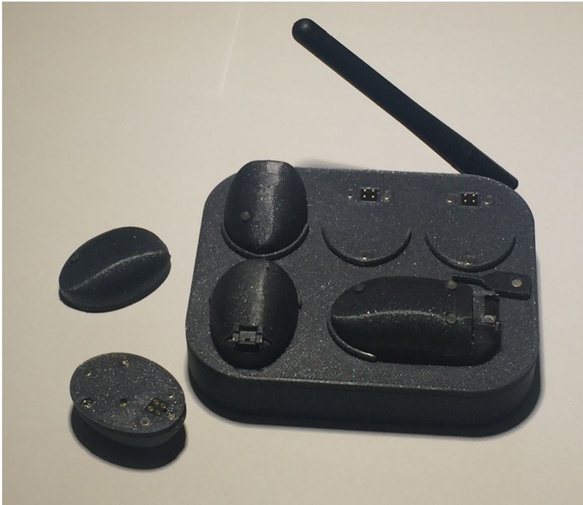
Figure 6.6: The completed hub and nodes. The Analog, Output, and IMU nodes can be seen with some docked and some undocked, showing both sides of the connectors. The dipole antenna is also displayed in the back.
