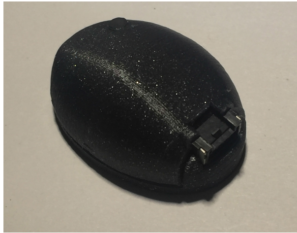
Figure 6.4: Attached to the back of the Analog node, the small 4 pin rectangular connector is almost completely embedded into the node, with no effect on its small form factor.
