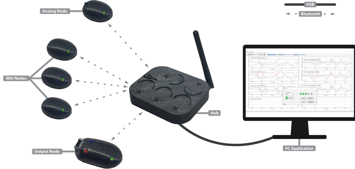
Figure 2.1: Overview of the system, including the nodes, hub, and PC application.
