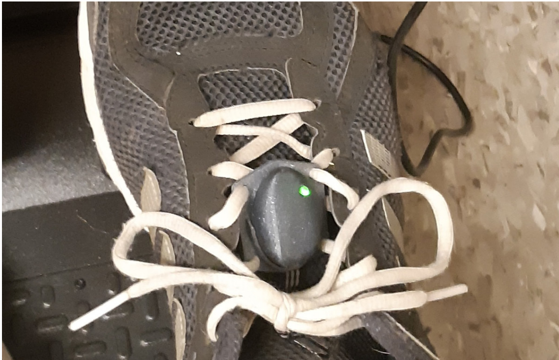
Figure 8.4: IMU node for measuring foot motion. This IMU node is attached to the shoelace snap anchor, which attaches to the shoe securely through the laces. This allows the easy removal of the node while maintaining a strong connection to the shoe even under intense motion.
