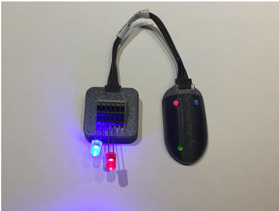
Figure 6.5: Output node connected to the terminal connection module, with the Blue and Red channels toggled on.
