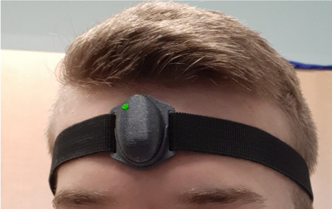
Figure 8.2: IMU node for measuring head motion. The node was connected to an anchor with a flexible strap, forming a comfortable and easy to wear headband.
