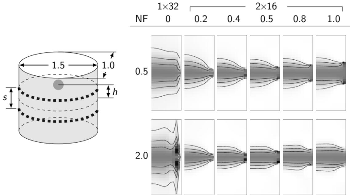
Plane separation  $s$ , vs. normalized amplitude response (sum of in-plane image pixels divided by the centre-slice value) in sagittal plane.
