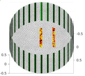
Using 32 equally spaced electrodes of the indicated width. Stimulation patterns were "skip 4" with monopolar voltage measurements on all electrodes (including driven ones).
