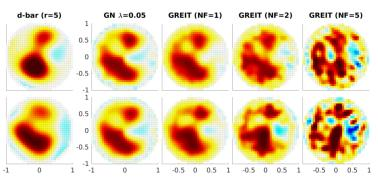
D-bar shows a different pattern (lower spatial frequency) for the reconstructed noise compared GN and GREIT.
