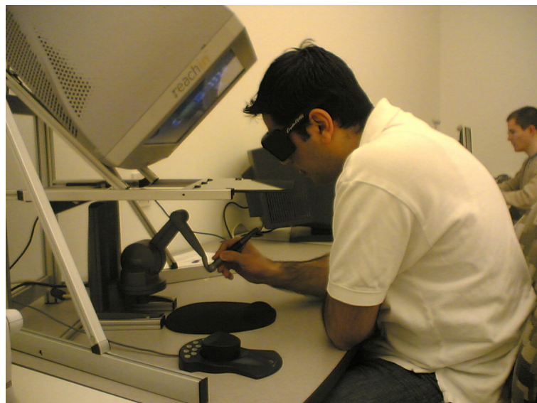
Figure 1 b. The PHANToM device used as the haptic instrument.
