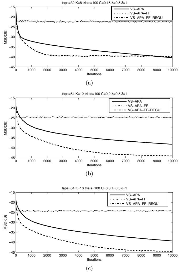
**Figure 3.** Comparisons among VS-APA, VS-APA-FF, and VS-APA-FF-REGU, G1 colorization.  $\lambda = 0.5$ . (a)  $K=8$ , taps=32,  $C=0.15$ ; (b)  $K=12$ , taps=64,  $C=0.2$ ; (c)  $K=16$ , taps=64,  $C=0.3$
