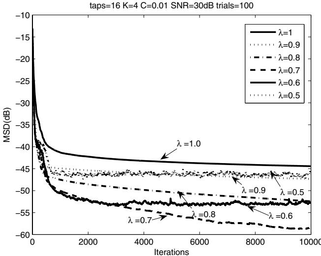
**Figure 1.** *MSD* vs. iteration number for *VS-APA-FF* for effect of different forgetting factors  $\lambda$ . ( $L=16$ ,  $K=4$ ,  $SNR=30dB$ , G2 colorization)
