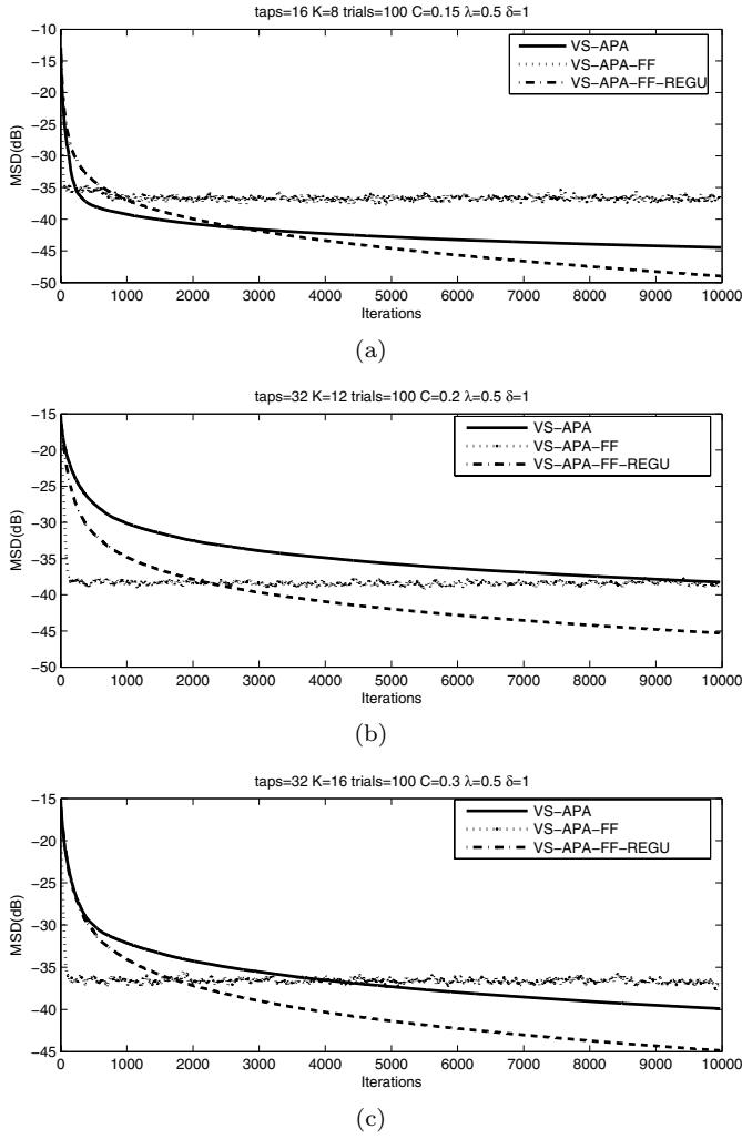
**Figure 2.** Comparisons among VS-APA, VS-APA-FF, and VS-APA-FF-REGU, G2 colorization.  $\lambda = 0.5$ . (a)  $K=8$ , taps=16,  $C=0.15$ ; (b)  $K=12$ , taps=32,  $C=0.2$ ; (c)  $K=16$ , taps=32,  $C=0.3$
