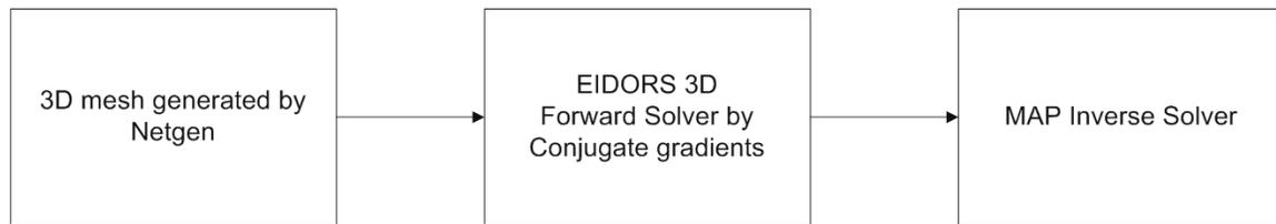
**Figure 4.6 Block Diagram for generating simulated data**
