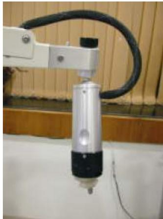
**Figure 7: 50 MHz transducer (taken from Deepak (2002))**
