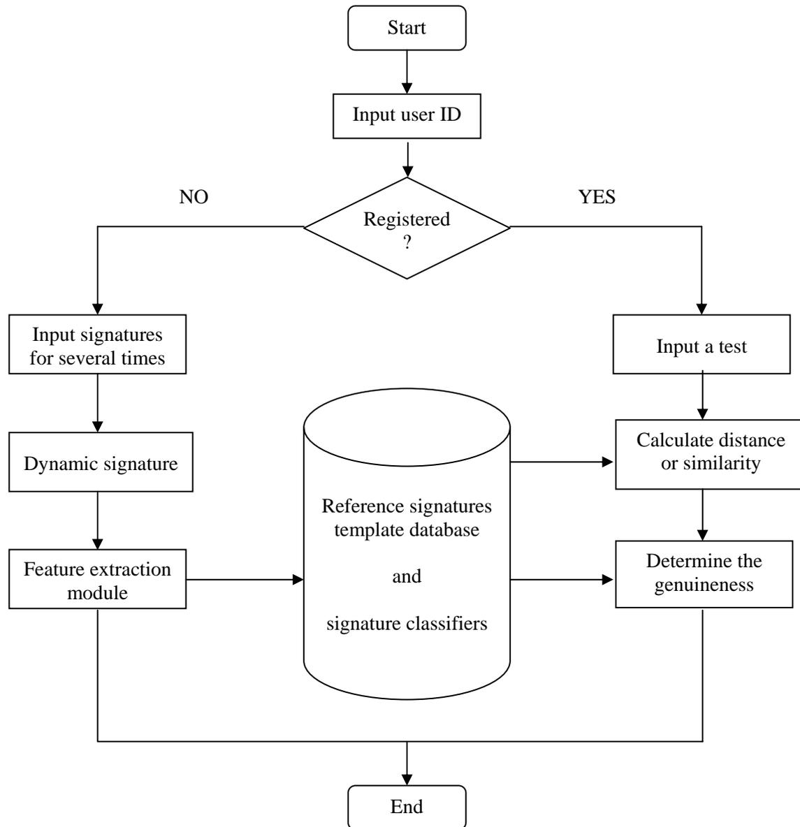
**Figure 1.1** A typical model for signature verification system.
