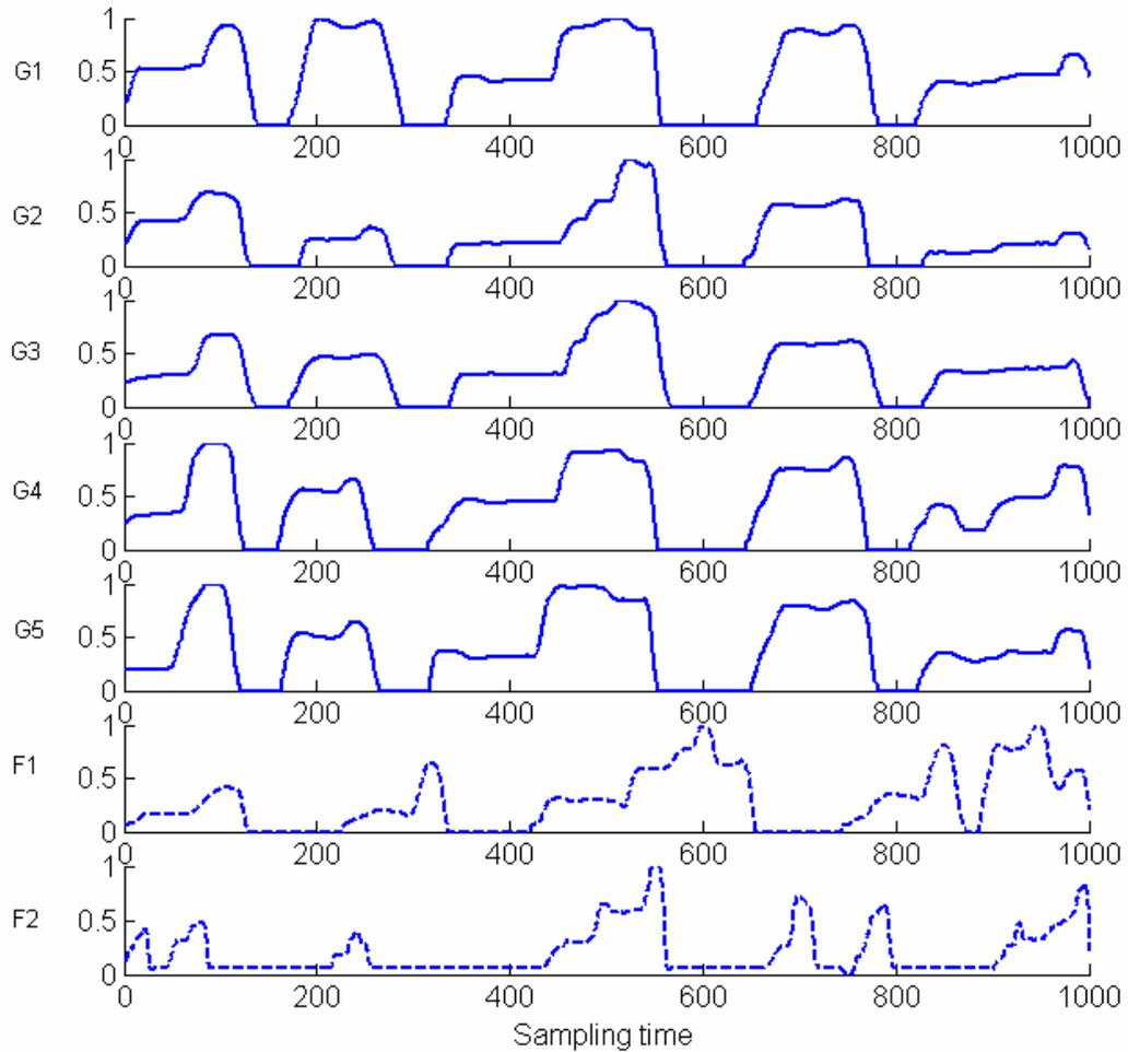
**Figure 4.12** Comparison of pressure stroke between genuine signatures and forgeries. (Stroke-based normalized pressure versus time of 5 genuine signatures and 2 forgeries. G1, G2, G3, G4, and G5 represent the pressure signals of the genuine signature while F1 and F2 refer to those of forgeries. The 4<sup>th</sup> stroke in each genuine signature is the significant stroke.)
