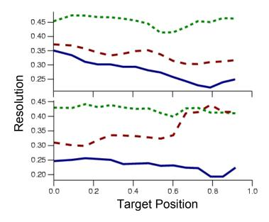
Resolution vs. target position for adjacent (lower) and opposite (upper) current patterns. Reconstruction matrices used are:  $\mathbf{B}_0$  (no electrode errors, solid line),  $\mathbf{B}_Z$  (electrode error data set to zero, dotted line), and  $\mathbf{B}_{\sigma=\infty}$  (electrode noise in regularized inverse, dashed line)
