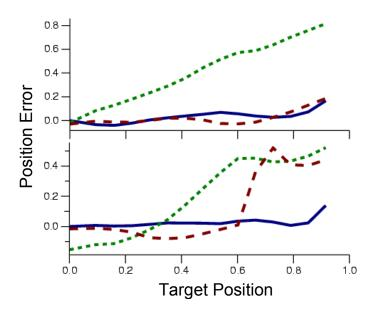
Position error vs. target position for adjacent (lower) and opposite (upper) current patterns. Reconstruction matrices used are:  $\mathbf{B}_0$  (no electrode errors, solid line),  $\mathbf{B}_Z$  (electrode error data set to zero, dotted line), and  $\mathbf{B}_{\sigma=\infty}$  (electrode noise in regularized inverse, dashed line)
