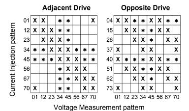
Block diagram of measurement patterns for an 8 electrode EIT system, using adjacent drive (left) or opposite drive (right). Current injection patterns are shown on the vertical axis, where a current applied between electrodes 1 and 5 is indicated 15.
