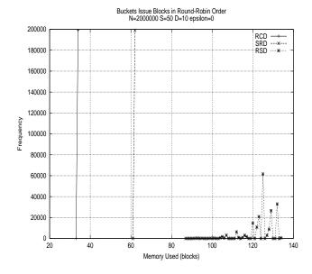
Figure 7: (Round-robin bucket order) The distribution of memory usage is shown for each variant except FRD when  $\epsilon = 0$ . The consumption of FRD was much larger and goes off the graph to the right. All of the variants tend to use more memory than when  $\epsilon = 0.1$ . RCD and SRD used a fixed amount of memory after steady state was reached.
