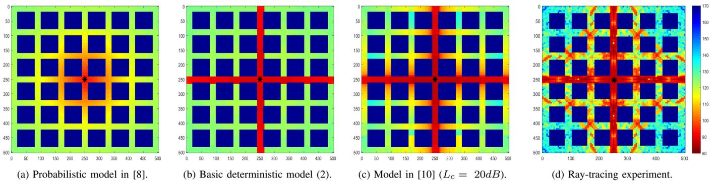
Fig. 2: Propagation patterns for a drone-BS at 200 m altitude.
