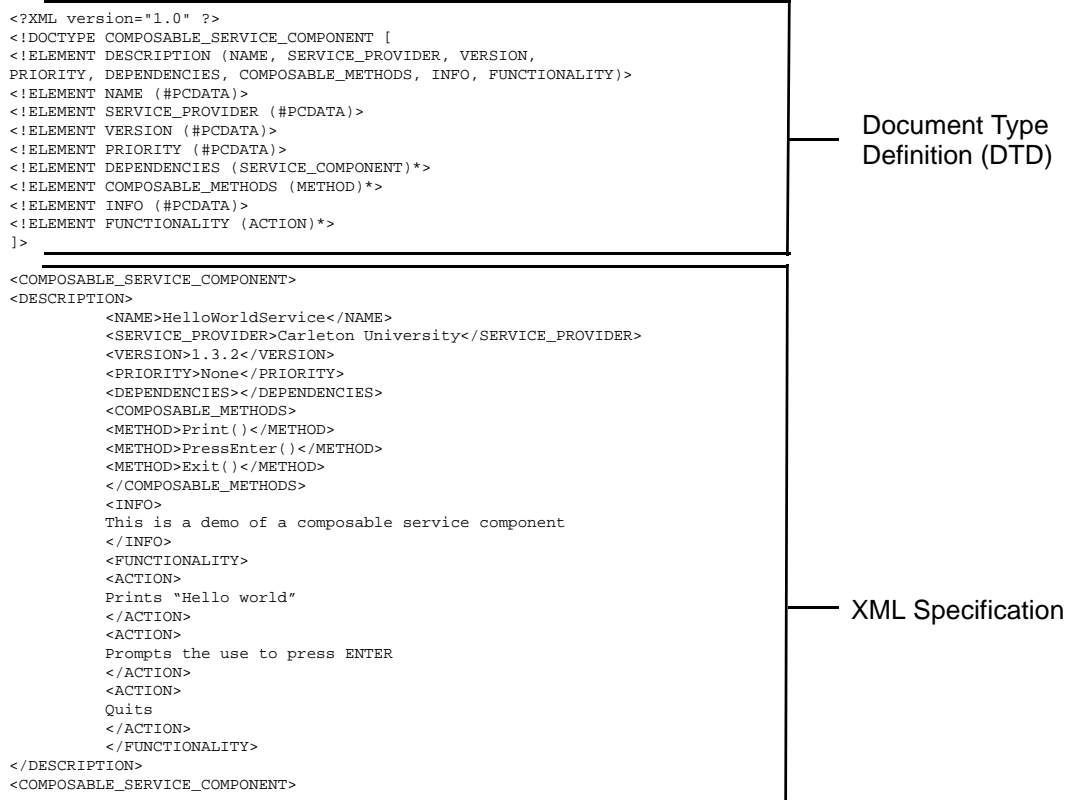
Figure 5.6: A Sample XML Service Component Specification
