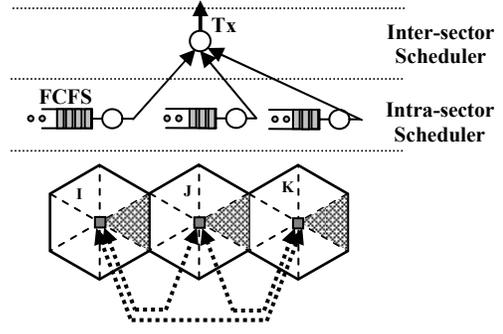
Fig. 2. Block diagram of the scheduling scheme in group  $\{I, J, K\}$ .
