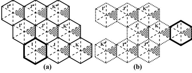
Fig. 1. (a) Nine-cell network, (b) wraparound interferer positions for SSs in BS  $I$ .
