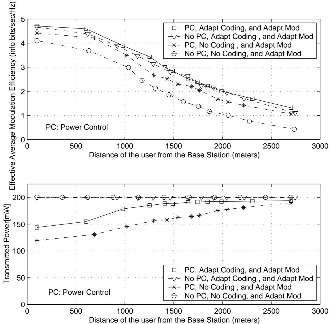
**Fig. 6: The impact of using combined adaptive modulation, power control, and adaptive coding on the system performance**
