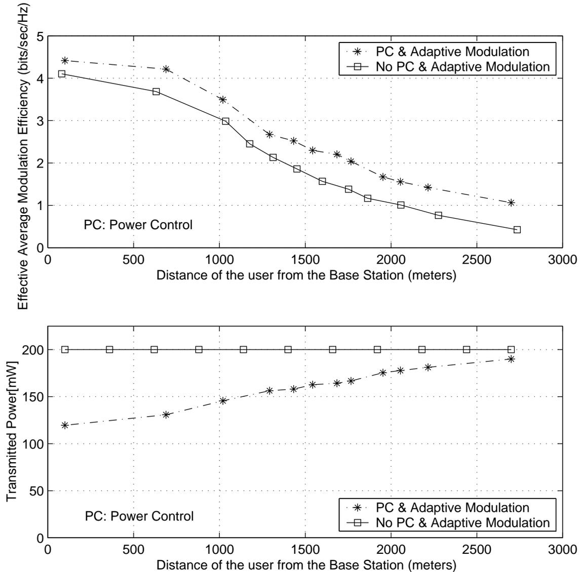
**Fig. 5: The impact of using combined adaptive modulation and power control on the system performance (no coding)**
