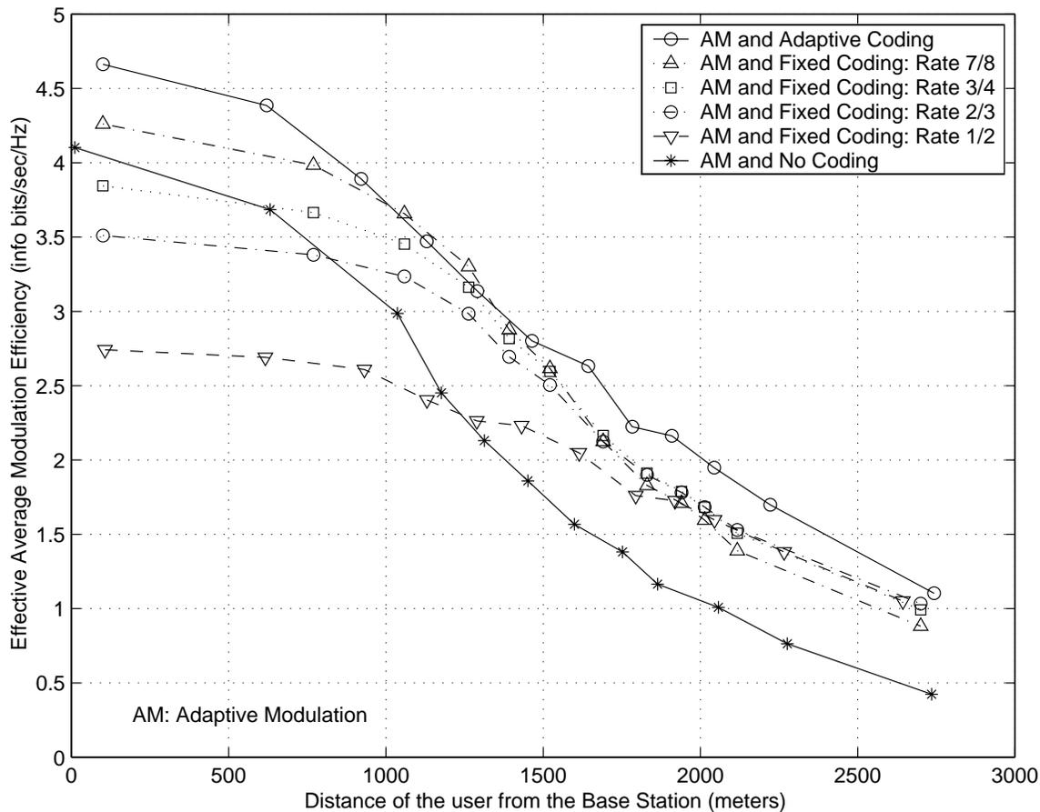
**Fig. 4: The impact of using combined adaptive modulation and adaptive coding on the system performance (no power control)**
