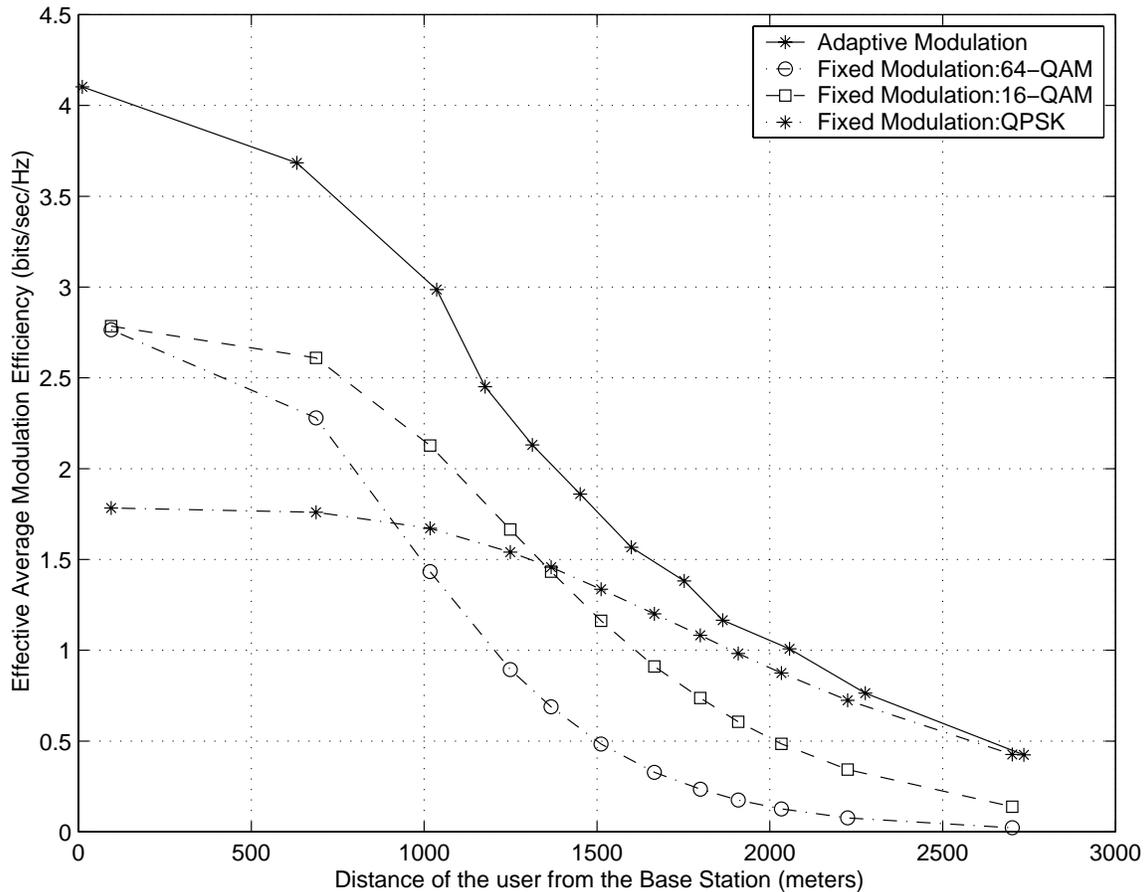
**Fig. 3: The impact of using adaptive modulation on the system performance (no coding, no power control)**
