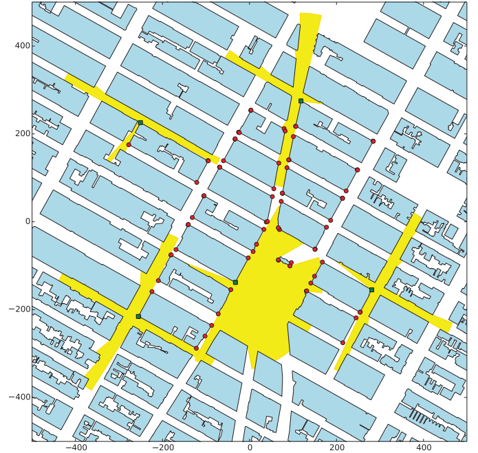
Fig. 3. WMBSs candidate locations (red dots) on a 1 \text{ km}^2 tile of Manhattan Island, NY (centre: 73.9909^\circ \text{W} , 40.7373^\circ \text{N} ), with r = 200 \text{ m} . We manually select a few of the candidate locations (green dots) and show their LOS regions (in yellow) to illustrate what typical LOS coverage regions may look like.
