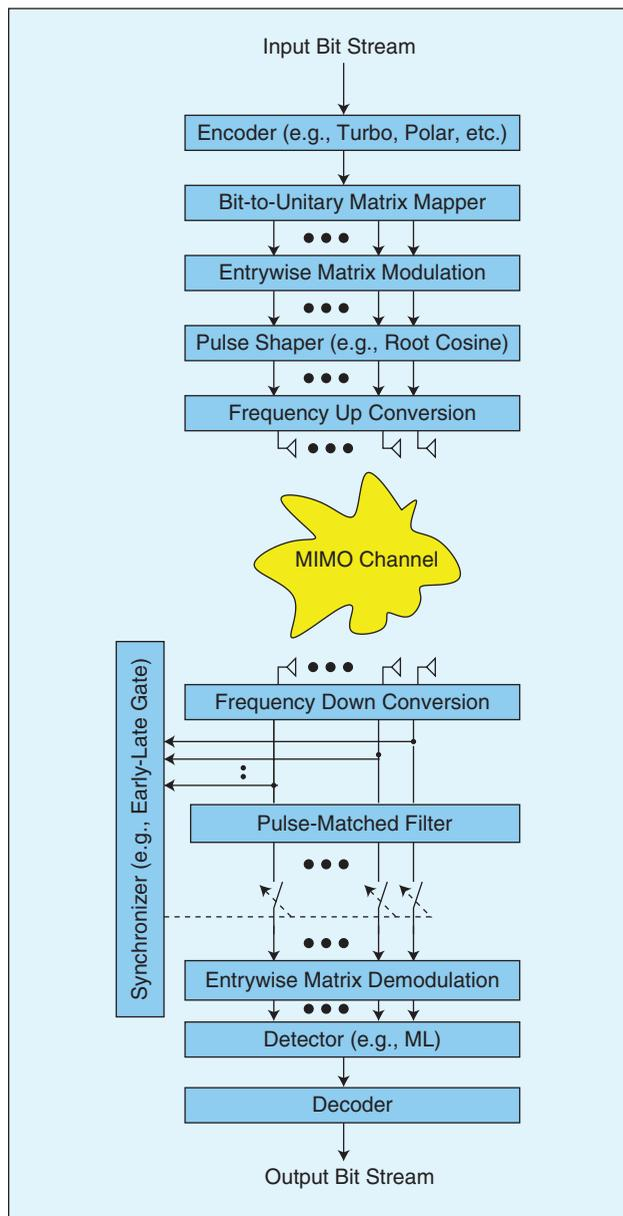
**FIGURE 5** The potential embodiment of a noncoherent system. ML: maximum likelihood.
