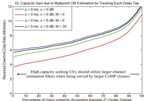
Fig. 4. Capacity increase due to multi-point channel estimation using CSI-RS.
