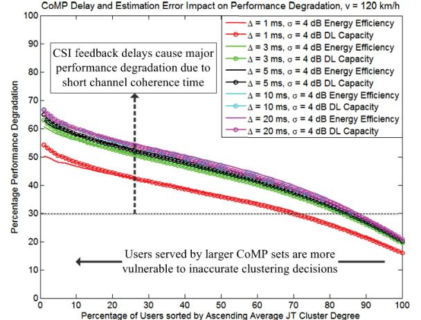
Fig. 3. CoMP joint transmission performance degradation in high mobility condition.
