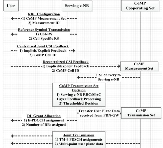
Fig. 1. Inter - eNB joint transmission DL CoMP procedures.
