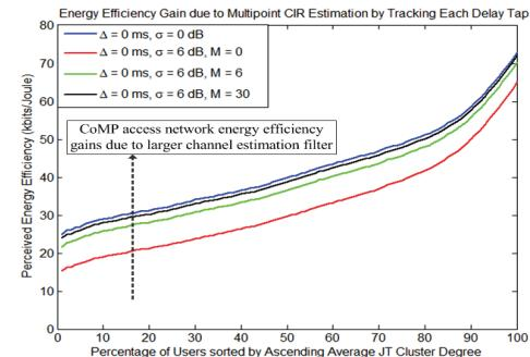
Fig. 5. Energy efficiency increase due to multi-point channel estimation using.
