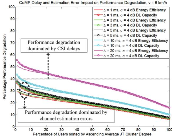
Fig. 2. CoMP joint transmission performance degradation in low mobility condition.
