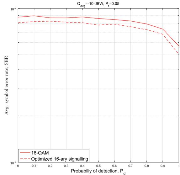
Fig. 4. Average SER for 16-ary signaling versus probability of detection ( $P_d$ ) in the SSS scheme.
