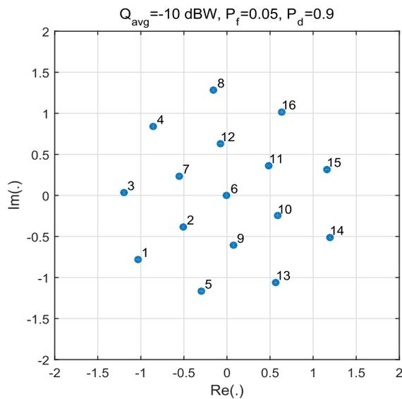
Fig. 6. Optimized 16-ary constellations for  $P_f = 0.05$ ,  $Q_{\text{avg}} = -10$  dBW, and  $P_d = 0.9$ .
