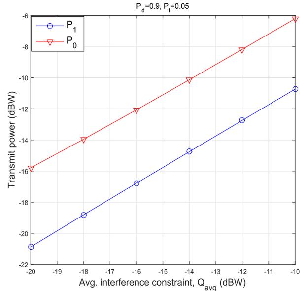
Fig. 3. Power allocation for 16-ary signaling versus average interference constraint ( $Q_{\text{avg}}$ ) in the SSS scheme.
