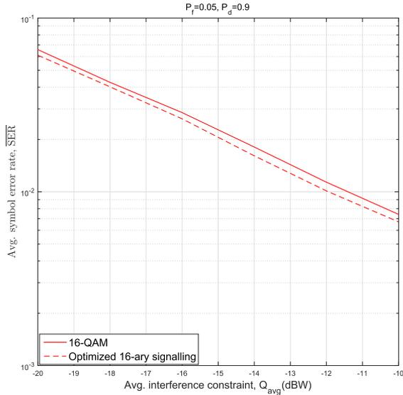
Fig. 2. Average SER for 16-ary signaling versus average interference constraint ( $Q_{\text{avg}}$ ) in the SSS scheme.
