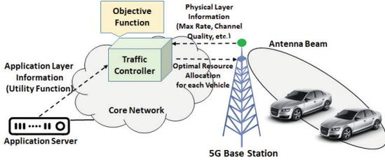
Fig. 2. Typical network-centric scenario and high-level system architecture.
