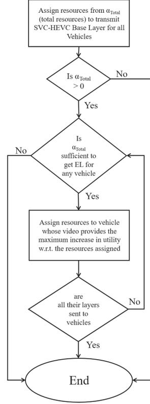
Fig. 4. The flowchart for assigning resources for base layer and enhancement layers (EL).
