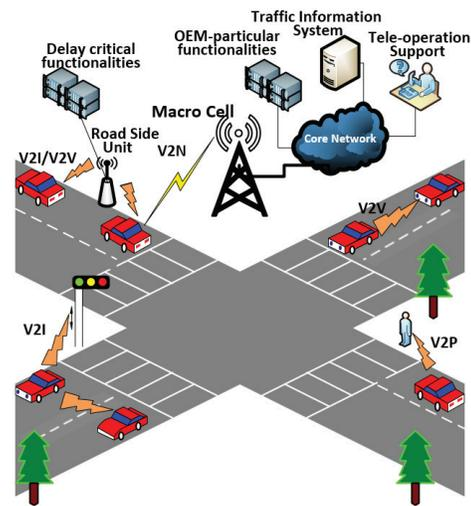
Fig. 1. Example of V2X deployment, transport options and services offering [Note: Here X represents V for vehicle, or N for Network, I for Infrastructure].
