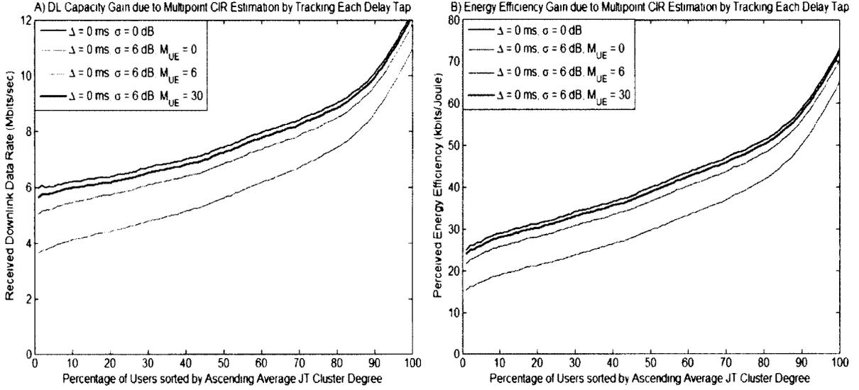
Figure 5.1: Downlink capacity and energy efficiency increases due to multi-point CIR estimation by tracking each delay tap.  $\tilde{h}_{n,i}(t, \tau_l)$ , individually using the delay-cross power density functions formulated in (5.23).
