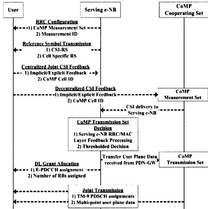
Figure 2.14: DL CoMP procedures for inter-eNB joint transmission schemes.
