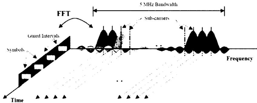
Figure 2.8: Time-Frequency domain representation of an OFDM signal shown in [28].
