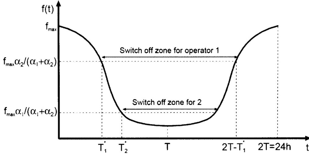
Figure 2.6: Cell switch off scheme enabled via cooperation among multiple network service providers shown in [22].
