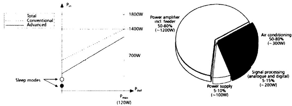
Figure 2.1: Power consumption distribution of radio access networks. adapted from [8] and [9].
