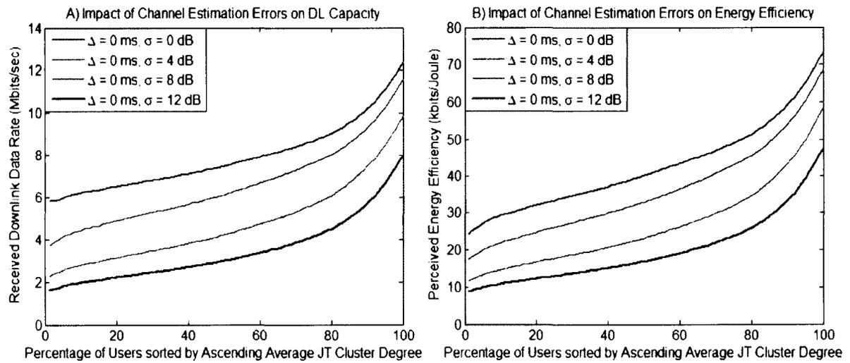
Figure 4.4: Downlink capacity and energy efficiency performance of CoMP schemes subject to channel estimation errors.
