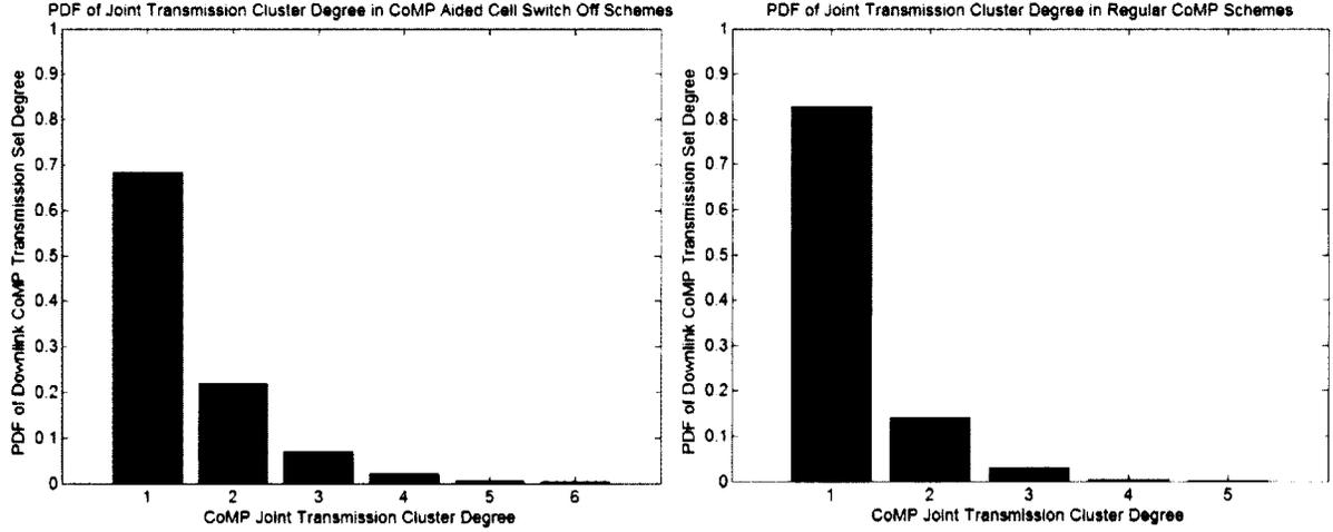
Figure 3.5: PDF of CoMP joint transmission cluster degrees for cell switch aiding versus regular CoMP schemes, simulated in stationary channels according to 3 dB clustering threshold.
