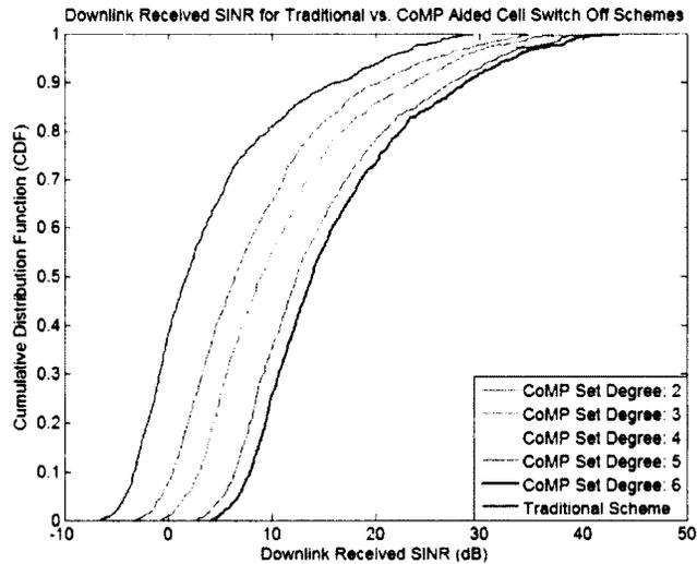
Figure 3.3: Received SINR CDF comparison between traditional and CoMP aided cell switch off schemes.
