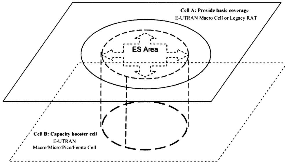
Figure 2.7: LTE cell switch off/on solution suggested in 3GPP release 8 workshops by [24].
