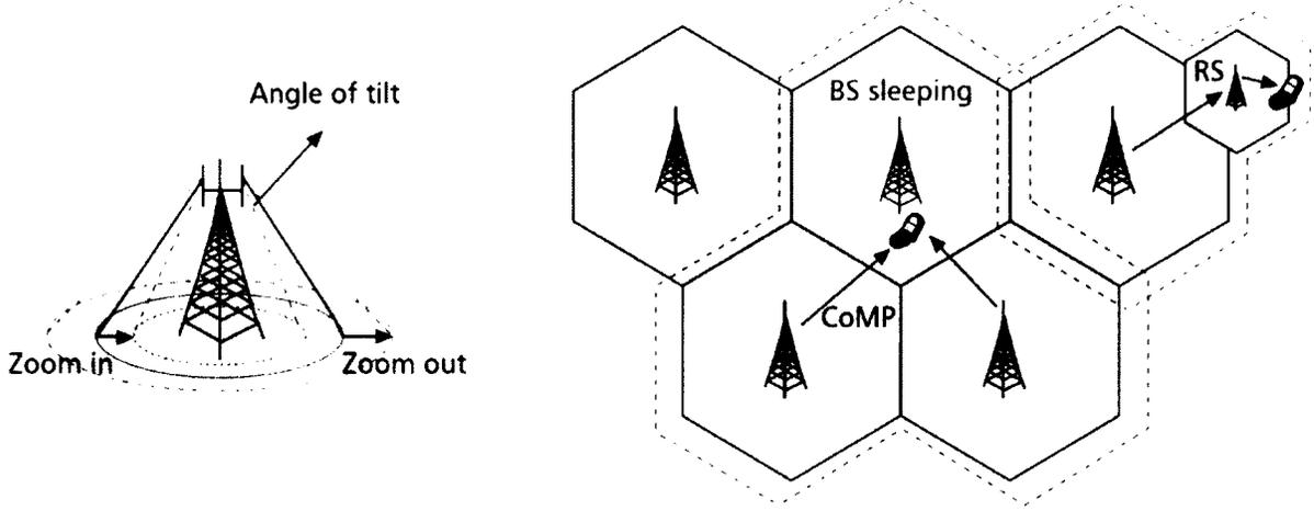
Figure 2.4: Low traffic cells switching off fully or zooming in while neighbor cells zoom out by antenna tilts. CoMP, or relaying approaches to serve the users located in the switched off cells as shown in [19].
