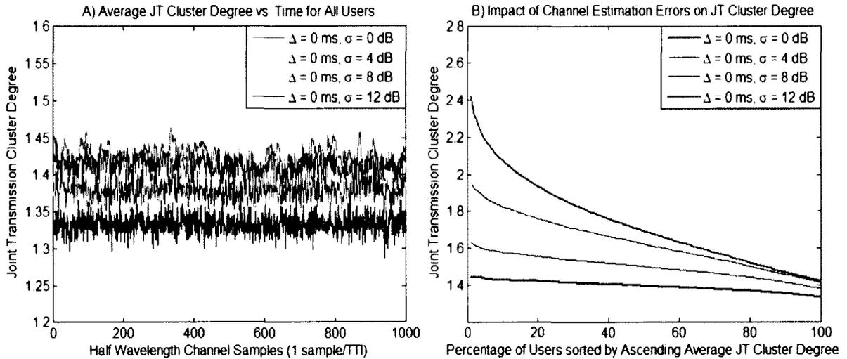
Figure 4.3: Joint transmission cluster degree changes due to channel estimation errors in fading channels.
