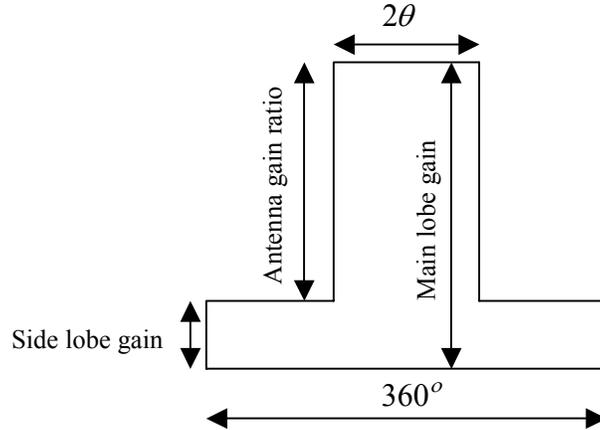
Figure 19: The gains of an ideal antenna
