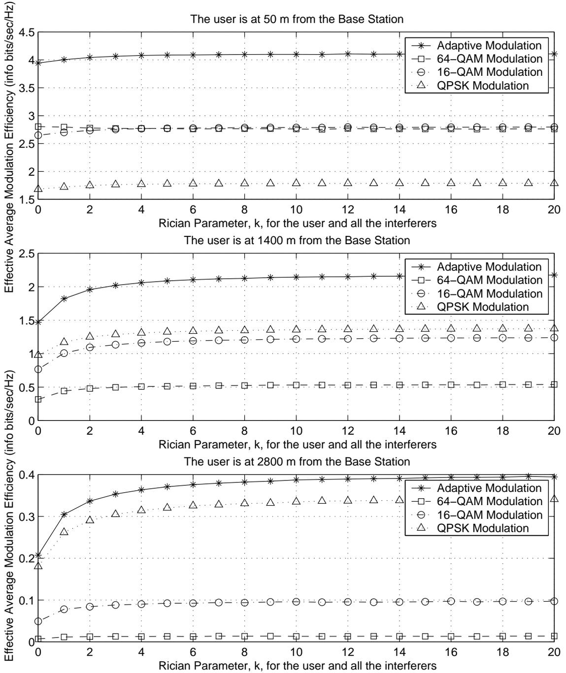
[Downlink transmission,  $f_c = 2.5$  GHz,  $BER = 10^{-5}$ ,  $T_x BW = 6$  MHz,  $T_x$  Power = 200 mW, Propagation exponent for the user and all the interferers = 4, Std. Dev. of log normal shadowing = 7 dB, Antenna beam width for the BS =  $90^\circ$ , Antenna beam width for the user and all the interferers =  $30^\circ$ , Antenna gains for the B.S, the user of interest, and all the interferers: Main lobe = 15 dB, Side lobes = -10 dB]
