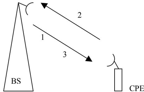
**Figure 2: A simplified model for implementing adaptive modulation in the downlink direction**
