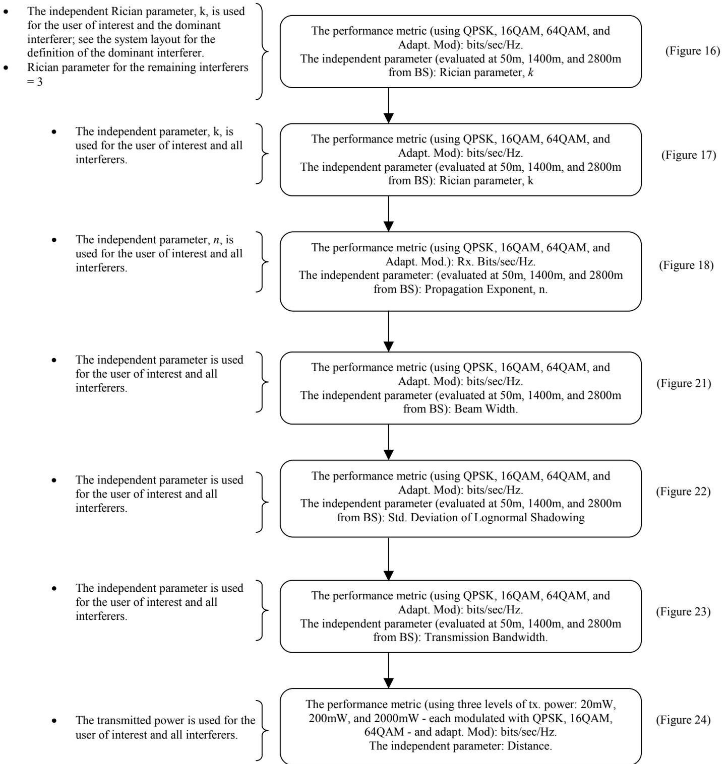
**Figure 15: The impact of various parameters on the system performance (the throughput)**
