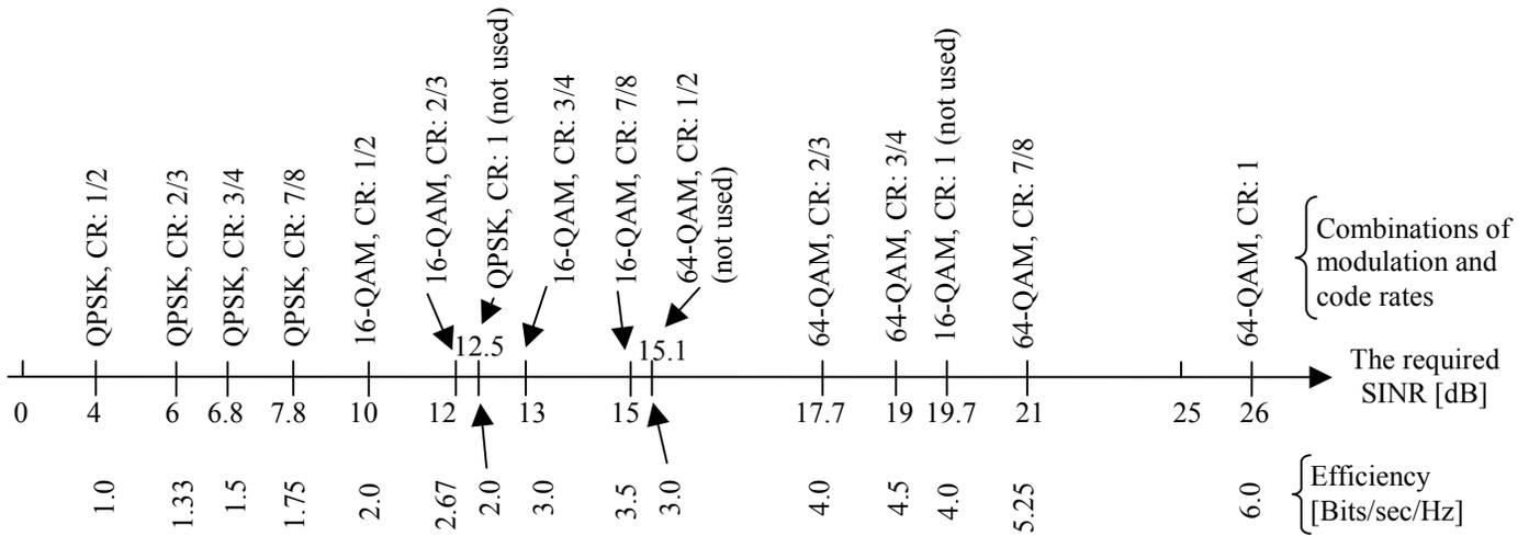
**Figure 29: Combinations of modulation and code rates and the corresponding number of received information bits that will yield BER of  $10^{-5}$**
