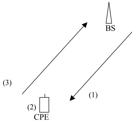
**Figure 5: A simplified model for UL open loop power control**
