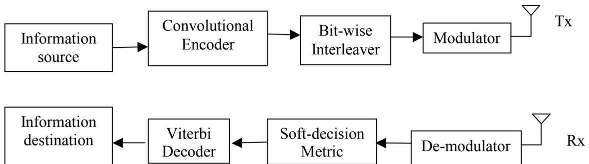
**Figure 3: Block Diagram for Bit-Interleaved Coded Modulation (BICM)**
