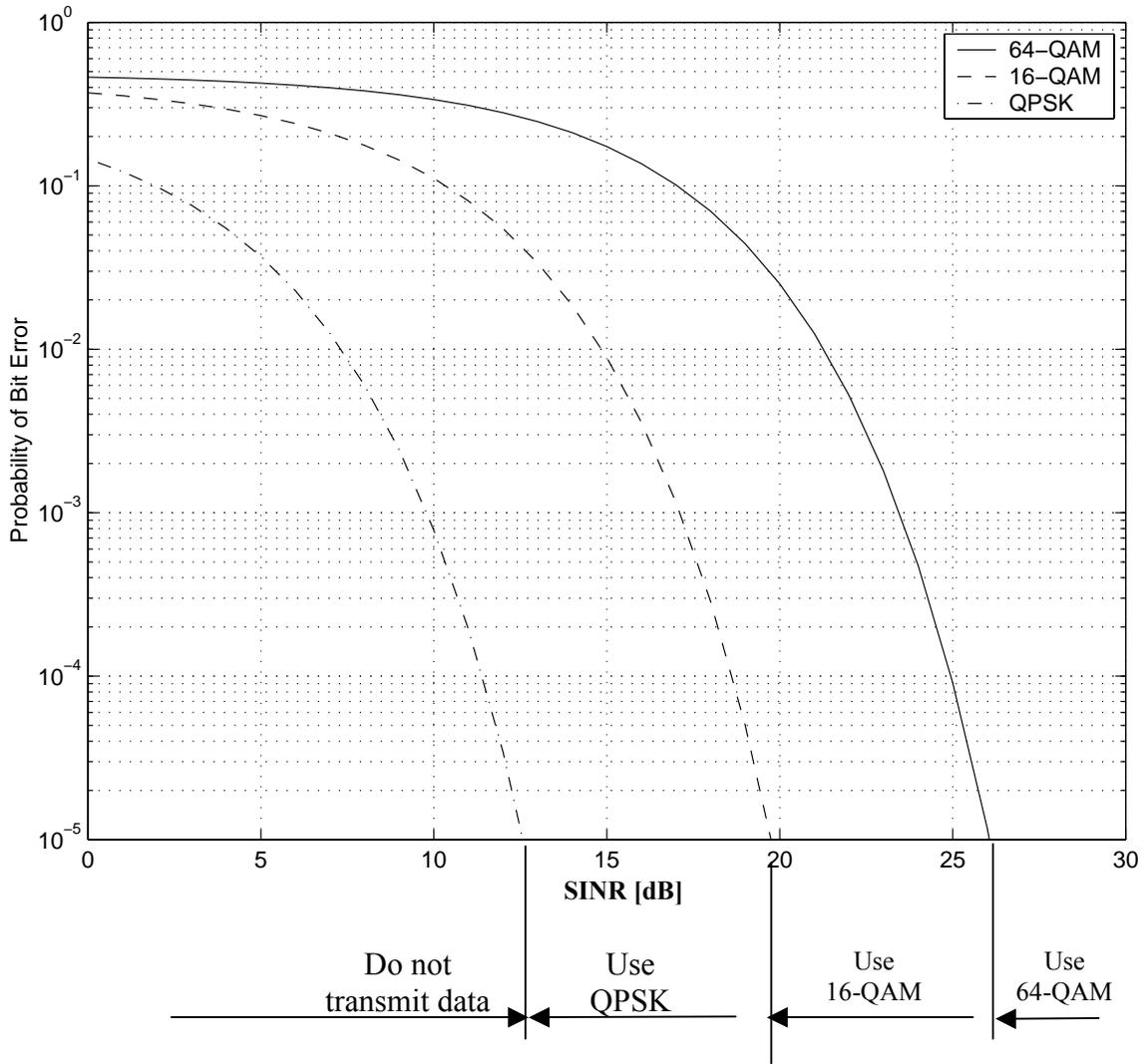
**Figure 1: An illustration of the implementation of adaptive modulation (assuming the noise plus the interference have Gaussian distribution)**
