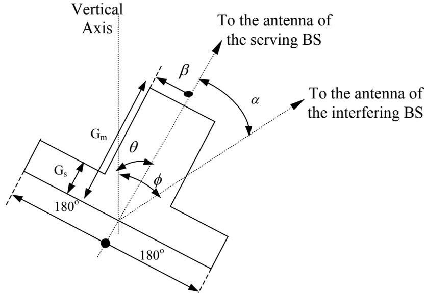
**Figure 11: The angle of arrival,  $\alpha$ , from the BS transmitter to the CPE's antenna centre**
