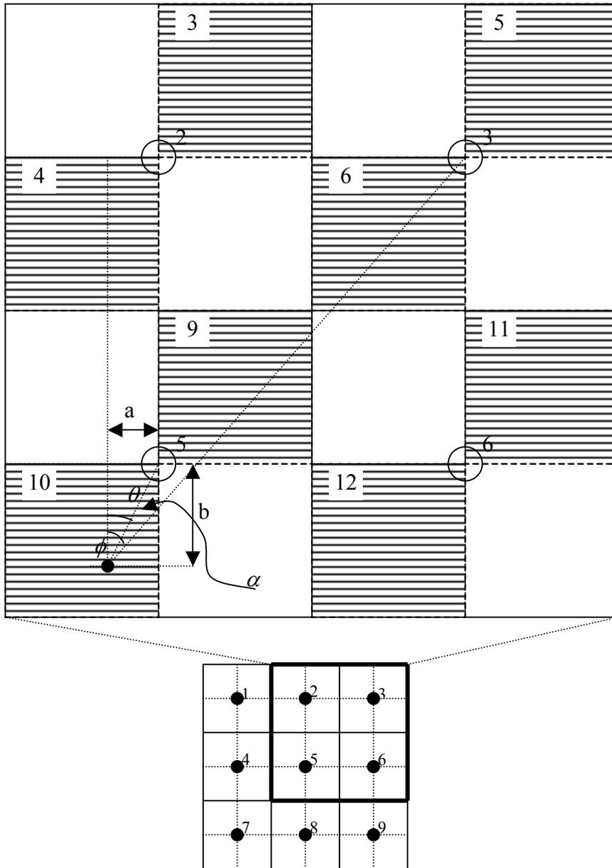
Figure 12: Evaluating the angle of arrival,  $\alpha$ , at the CPE's antenna
