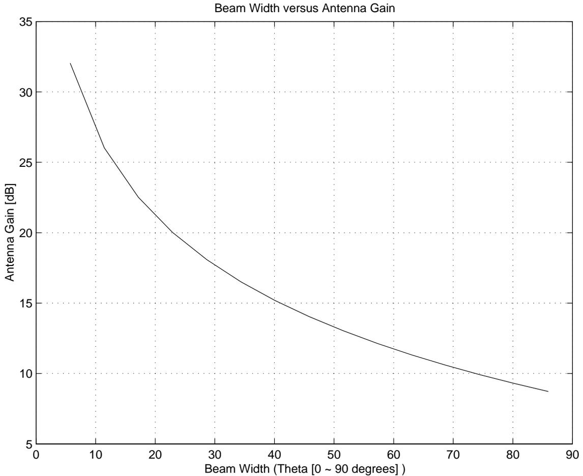
**Figure 20: The impact of the beam width on the antenna gain.**
