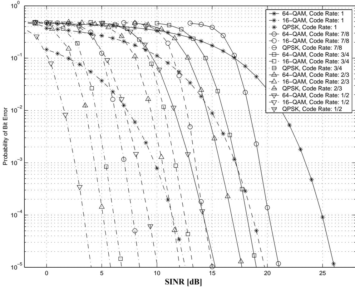
**Figure 28: Probability of Bit Error for several combinations of code rates and modulations<sup>2</sup> (assuming the noise plus the interference have Gaussian distribution)**
