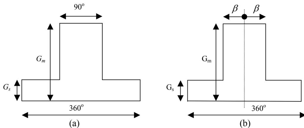
**Figure 10: The antenna beam widths and gains for (a) the base station and (b) the user equipment**
