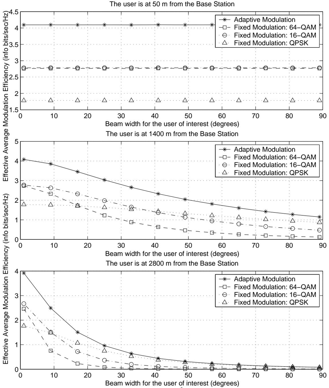
[Downlink transmission,  $f_c = 2.5$  GHz,  $BER = 10^{-5}$ ,  $T_x BW = 6$  MHz,  $T_x Power = 200$  mW, Rician parameter for the user of interest and the dominant interferer = 8, Rician parameter for the remaining interferers = 3, Propagation exponent for the user and all the interferers = 4, Std. Dev. of log normal shadowing = 7 dB, Antenna beam width for the BS = 90°, Antenna gains for the B.S, the user of interest, and all the interferers: Main lobe = 15 dB, Side lobes = -10 dB]
