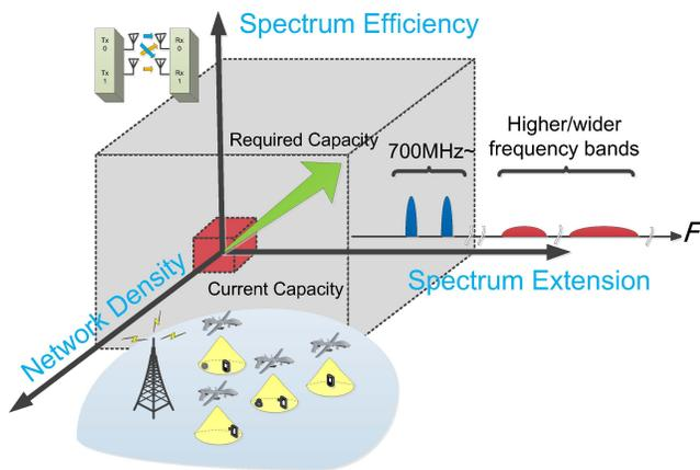
Fig. 3. Technical routes of improving the capacity of UAV networks.
