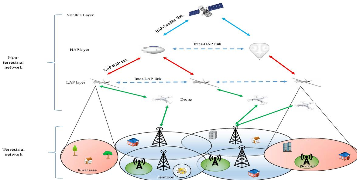
Fig. 1. An architecture of airborne communication networks.
