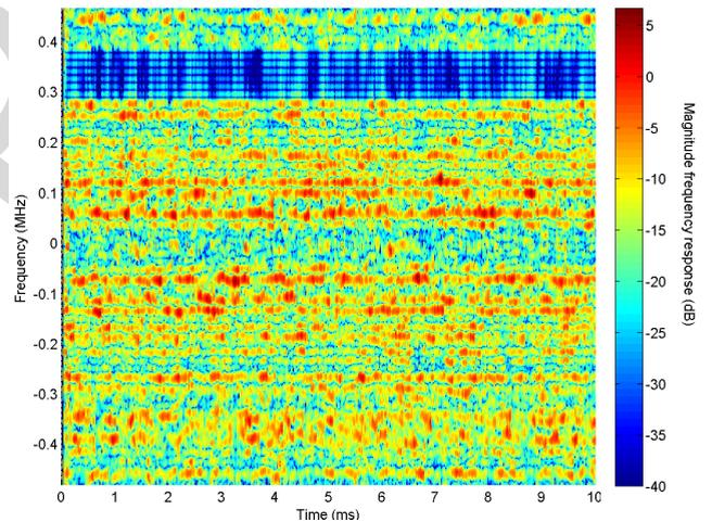
633 **FIGURE 4. Frequency response of the adaptive LCMV filter over the duration of one LTE frame (partial band interference scenario).**
