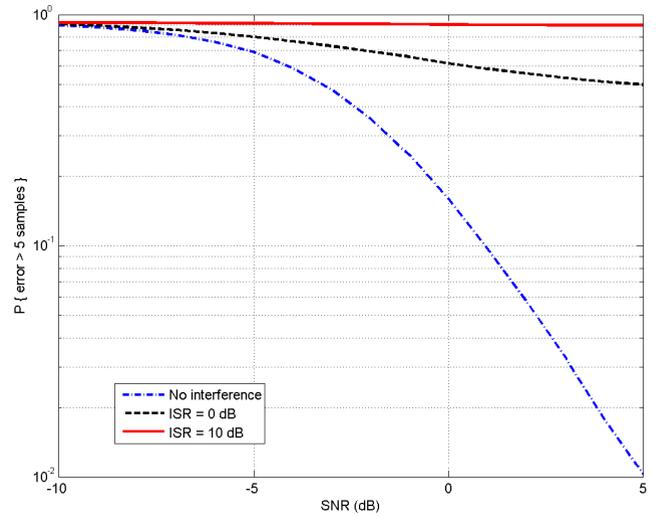
313 **FIGURE 2. Probability of error in finding the location of the OFDM symbol**
