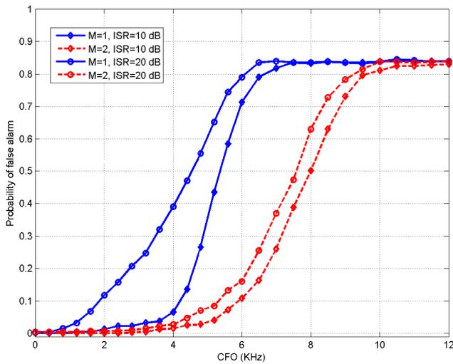
FIGURE 12. Probability of false alarm versus CFO.
