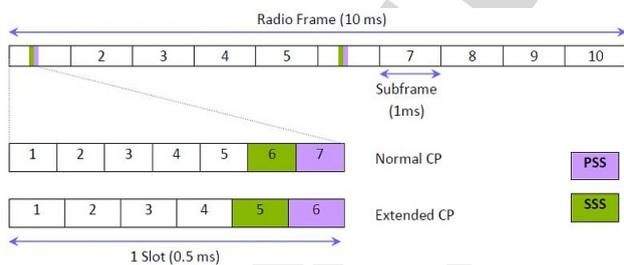
199 **FIGURE 1. Synchronization signals in LTE FDD downlink.**
