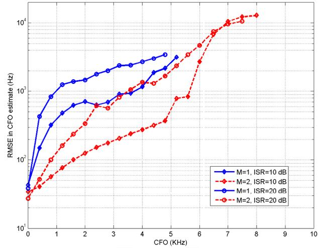
FIGURE 13. RMSE in CFO estimate versus CFO.
