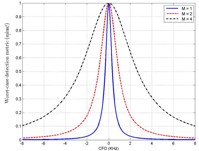
860 **FIGURE 14.** Sensitivity of detection metric  $u_i^*$  towards CFO for different
