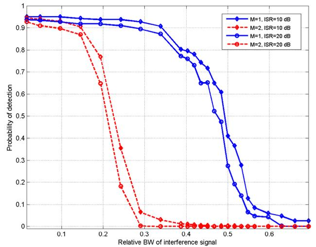
749 **FIGURE 9.** Probability of detection versus the relative BW of the
