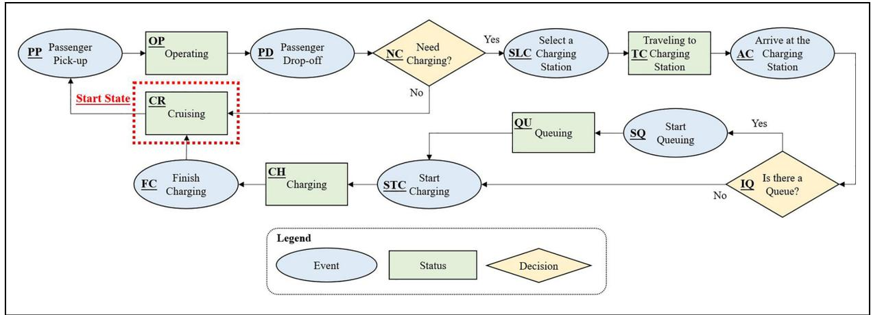
**Figure 4.** Flowchart of electric taxis' traveling and charging behaviors in the ABS model.
