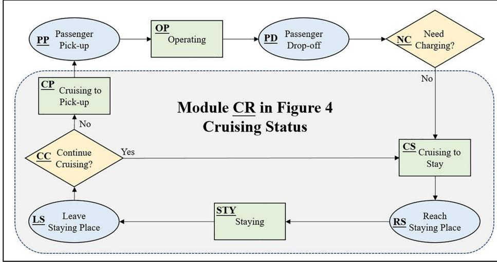
**Figure 6.** Flowchart of subprocesses in cruising status (Module CR in Figure 4).
