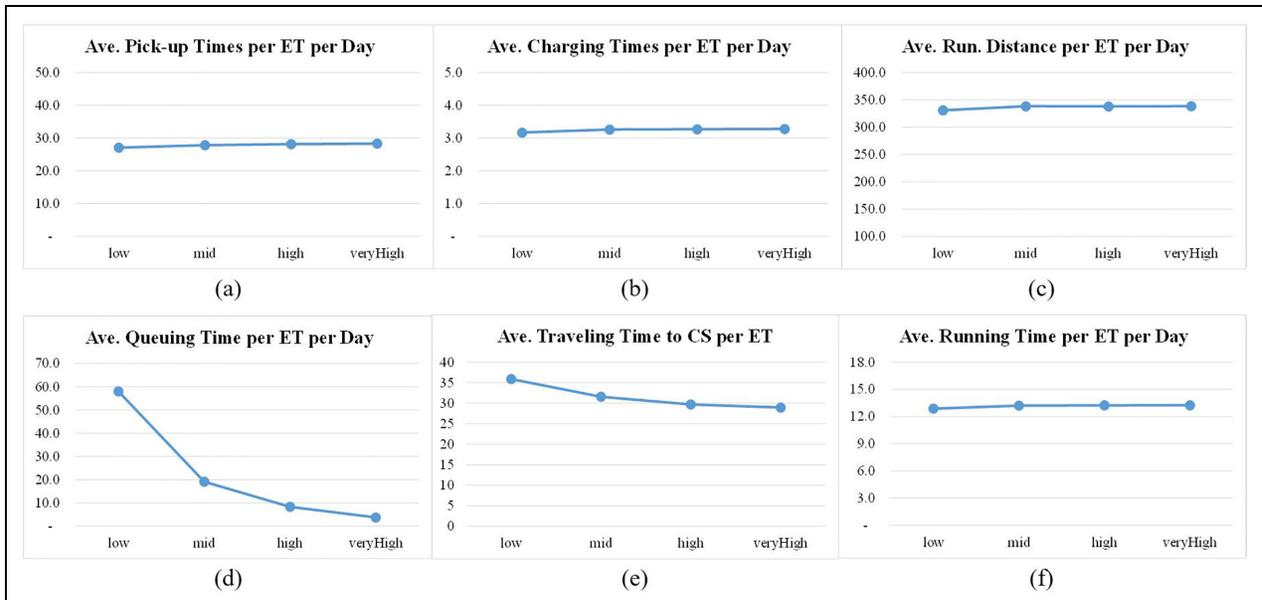
**Figure 14.** Sensitivity analysis for the charging pile volume in the ABS model. The label of y axis for subplot (a) Ave. pick-up times per ET per day; (b) Ave. charging Times per ET per day; (c) Ave. running distance per ET per day (kilometers); (d) Ave. queuing time per ET per day (minutes); (e) Ave. traveling time to CS per ET (minutes); (f) Ave. running time per ET per day (minutes).
