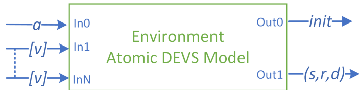
Fig. 8.1 The DEVS environment atomic model with its two input ports In_0 and In_1 used to receive the action a from the Agent DEVS model and the message [v] from the generators. The two output ports Out_0 (resp. Out_1 ) are used to send the initial message (resp. (s, r, d) ) to the Agent model.
