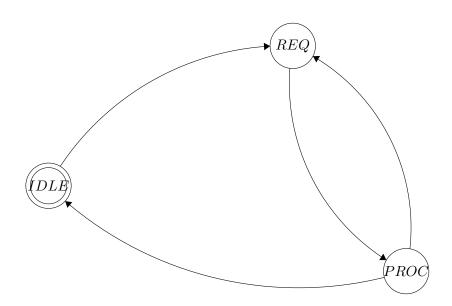
The finite state machine depicted above shows the states of a logic process during the rollback signaling phase in which the processing thread is asked to empty both the high and the low priority channels. This is a control system required to avoid unwanted rollback instances overlaps.
