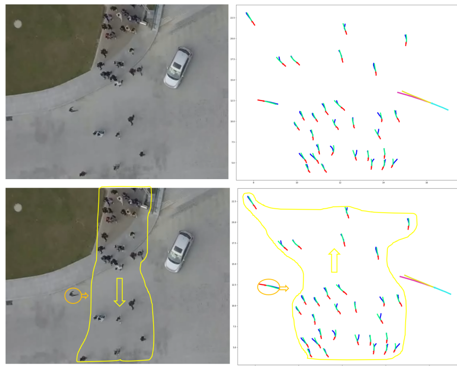
Figure 11. The output trajectories of the model on the 2nd scenario of the DUT dataset. Left: Visual of the scene. Right: Trajectory model and prediction. Pedestrians: red (observed trajectory), blue (ground truth), and green (predicted trajectory). Vehicles: turquoise (observed trajectory), yellow (ground truth), and pink (predicted trajectory). In the lower image, objects distinguished by a specific color are enclosed within a drawn outline and an arrow that indicates the direction of movement.
