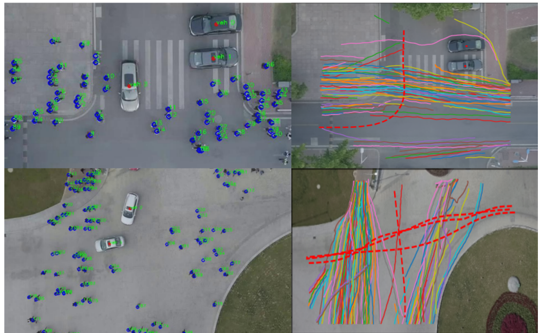
Figure 8. VCI-DUT Dataset with trajectories of vehicles (red dashed lines) and pedestrians (colorful solid lines). Upper: Intersection. Lower: Roundabout [33].
