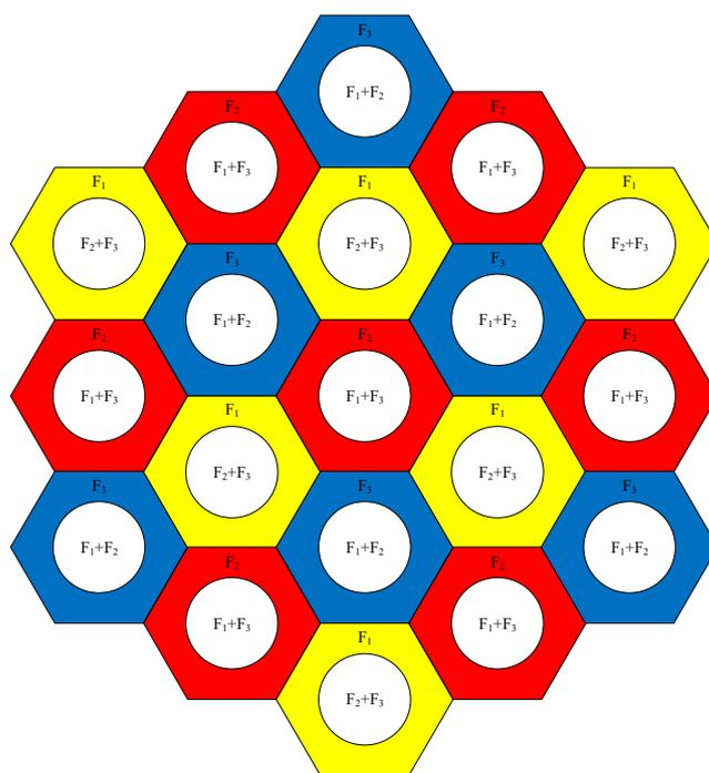
**Figure 2.** Deployment of base stations and channel assignment.
