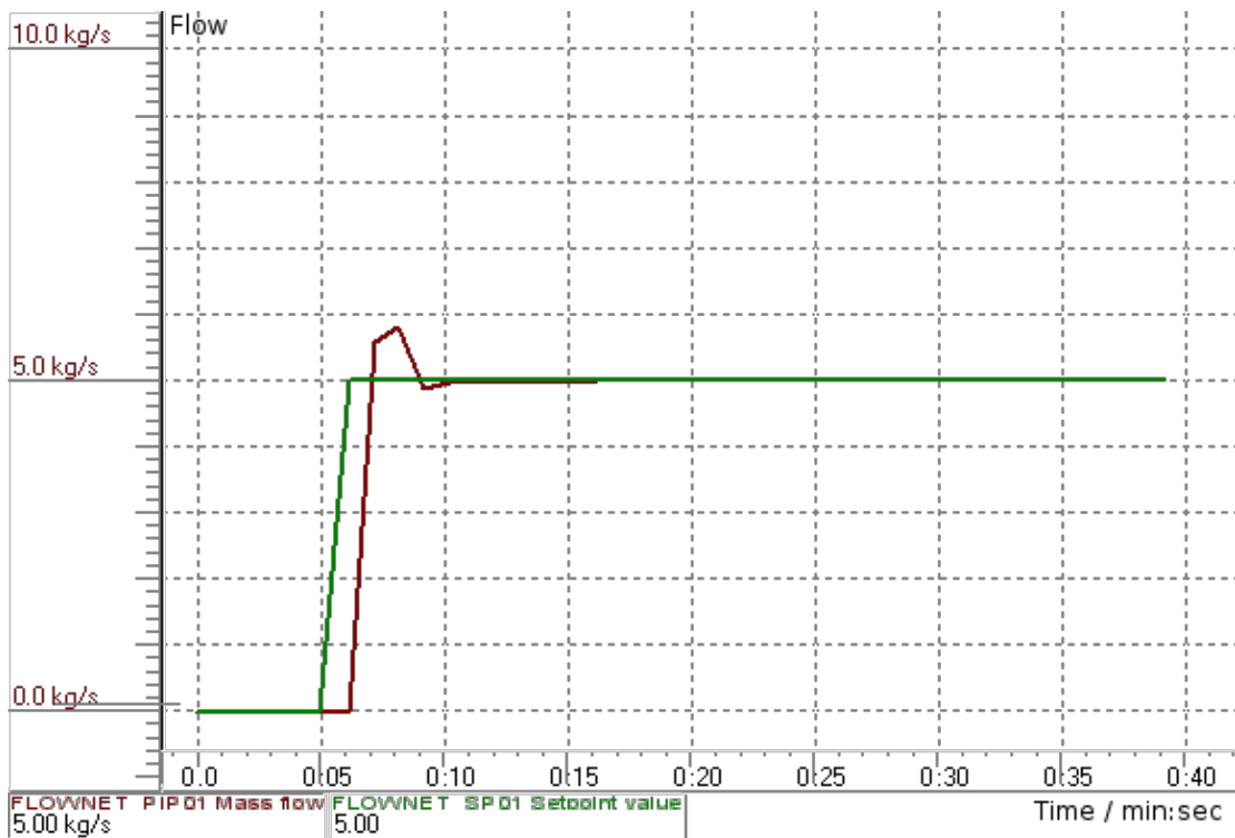
Figure 7.2: The step response of the simulation with the whole model simulated in Apros
