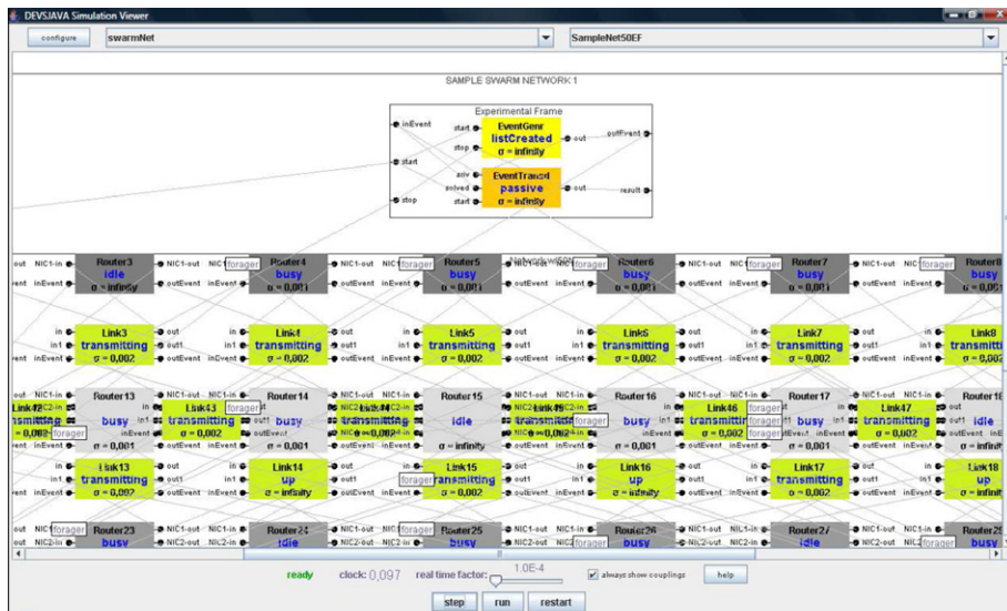
(a) 50 routers coupled network model without clustering and its experimental frame
