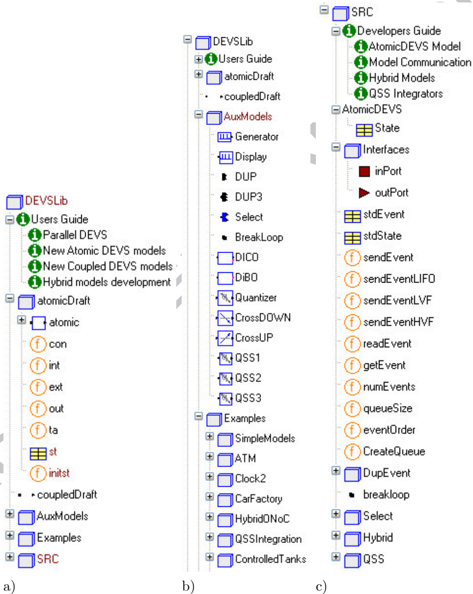
Fig. 1. DEVSLib library architecture: a) general architecture; b) user's area; and c) developer's area.
