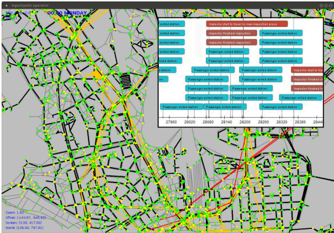
Fig. 4: High-level view of a running AgentPolis simulation model. Road (black), pedestrian (grey), tram (yellow) and metro (red) networks and UrbanCitizen (green) and PTDriver (yellow) agents are shown. Simulation events are depicted in the overlay window.
