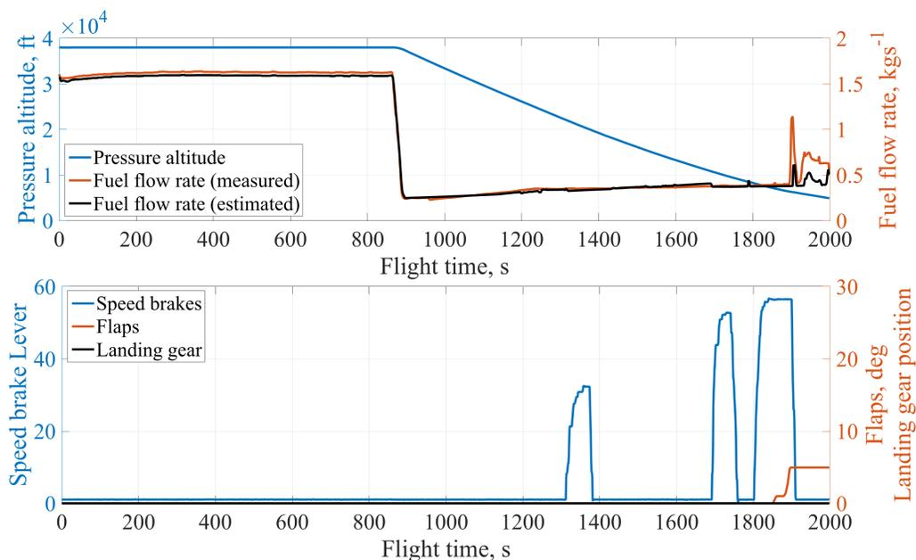
Figure 4: Fuel flow rate estimation and related time histories for Flight 35 (Top: Pressure altitude, measured fuel flow rate and estimated fuel flow rate. Bottom: Speed brake lever, flaps and landing gear).
