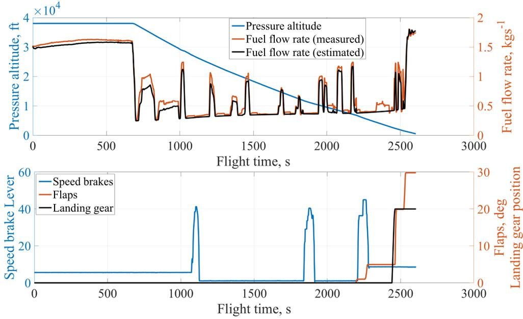
Figure 5: Fuel flow rate estimation and related time histories for Flight 15 (Top: Pressure altitude, measured fuel flow rate and estimated fuel flow rate. Bottom: Speed brake lever, flaps and landing gear).
