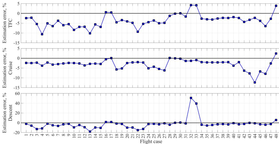
Figure 8: Estimation error of fuel consumption (Top: TFC. Center: Cruise phase. Bottom: Descent phase).
