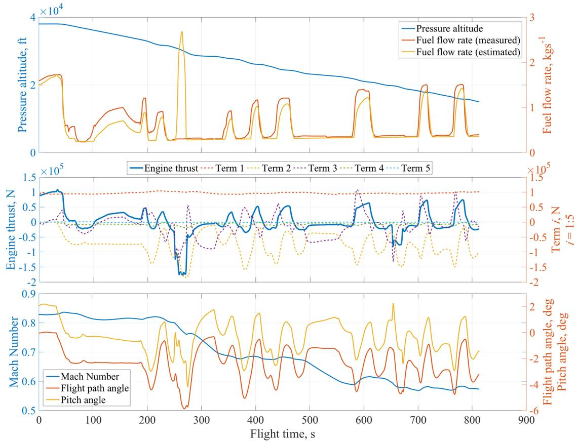
Figure 9: Time histories of performance parameters in Flight 4 (Top: Pressure altitude, measured and estimated fuel flow rate. Center: Thrust components. Bottom: Mach Number, flight path angle and pitch angle).
