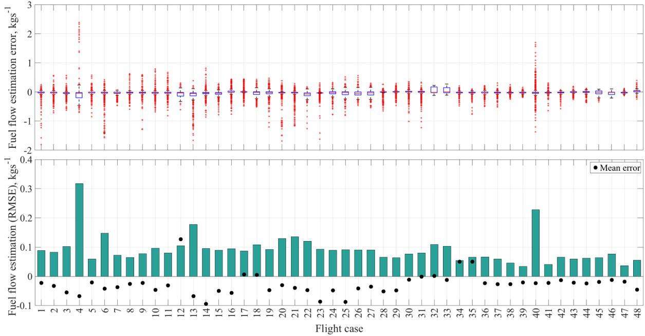
Figure 6: Estimation error of fuel flow rate (Top: Boxplot presentation. Bottom: Root Mean Squared Error (RMSE) and Mean error).
