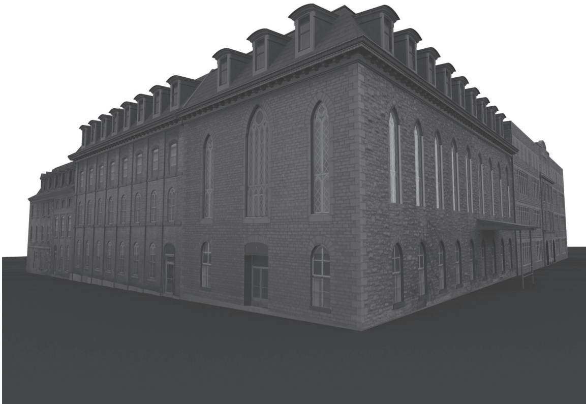
External building views were captured through a combination of photogrammetric and 3-D modeling techniques from archival photographs.
