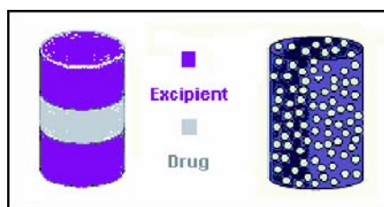
Figure 2: Layered compact versus matrix compact
