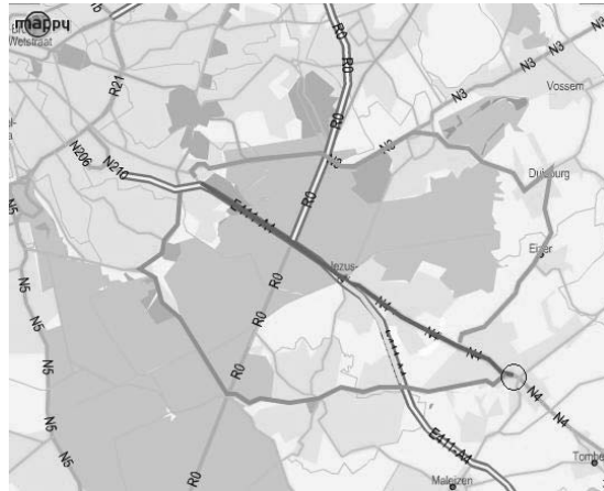
FIGURE 4.6 A car at the circle (at the bottom right) has three possible routes: straight ahead, left, and straight on and then right. In the current situation, the car follows the route straight ahead, which has the minimal cost.
