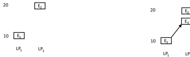
(a) LPs 1 and 2 have processed all events up to E_1 and E_2 respectively (b) E_1 schedules an event before E_2
