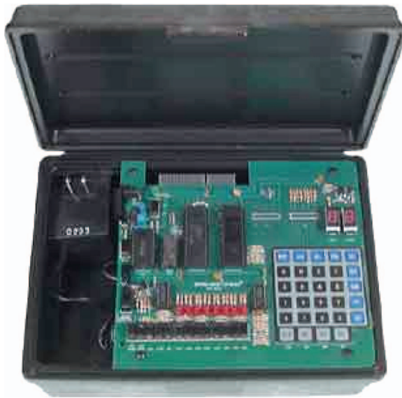
Figure 5. The 8085 hardware kit
