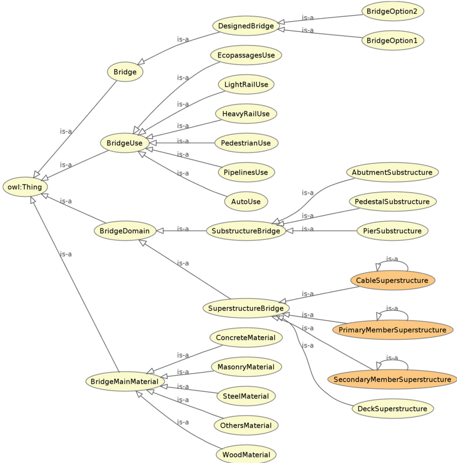
Fig. 1. Example of an ontology that conceptually models the different components of a bridge.
