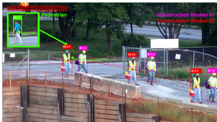
(b) Monitoring an unsecured construction gate (video processed results displayed as a time-lapse)
