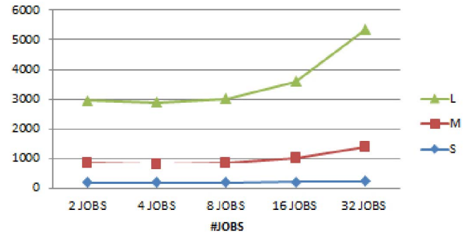
Figure 6. Response time (in seconds) for Small (S), Medium (M) and Large (L) size simulator instances for static configuration of simulator
