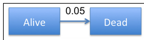
Figure 1. State transition diagram of a simple Markov model. The model uses two disease states, alive and dead , where the dead state terminates simulation. The yearly probability of transition between alive and dead states is 0.05.
